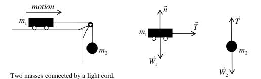
**Fig. 2**: Free- body diagrams for the two masses:
