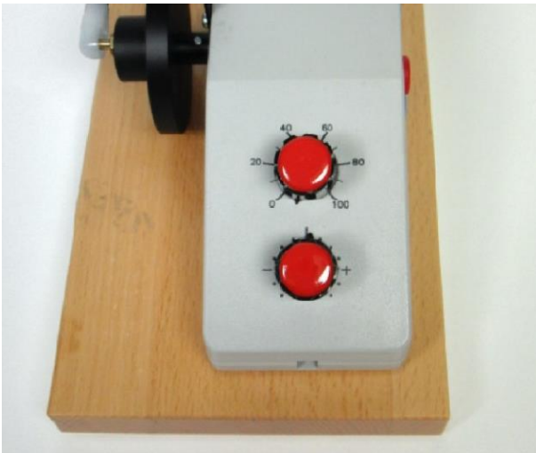
Figure 5. Control knobs to set the motor potentiometer. Upper knob: “coarse”; lower knob: “fine”.
